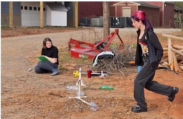
Shannon O'Connor's high school Physical Science completed a stomp rocket lab last week. Phoenix Blackwood's rocket flew about 56 feet in the air. In this lab, students measured the center of pressure and center of mass for their rocket designs, created fins and attached a nose cone in order to ensure stable flight. Students measured the angle of the highest point of the rocket with 2 observers and used a bit of trigonometry to determine how high the rockets flew.
