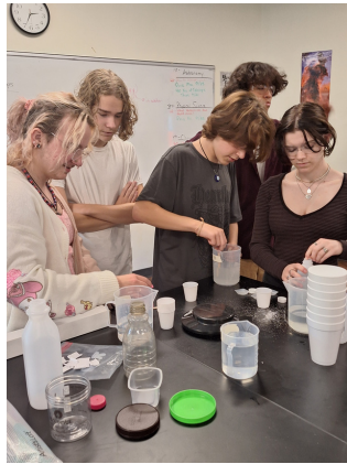
High school Chemistry students investigated the physical characteristics of the "Big 6 Plastics", which are types of synthetic polymers (the 6 main recycling numbers). Using three solutions of different compositions differing densities, they found the density of those plastics.
